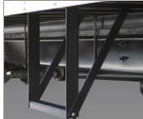
Side door step with brace
