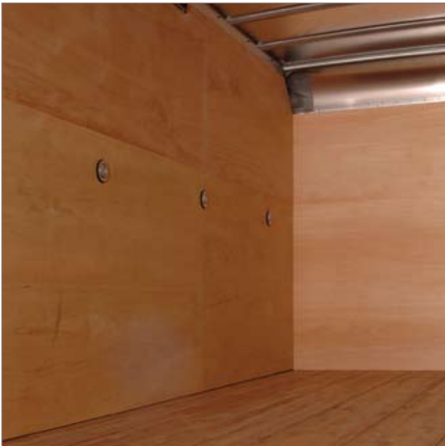
Full plywood liner with tie-rings
